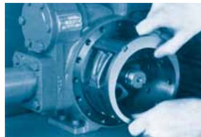
Easily replaceable liner restores efficiency.
