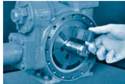
Simple vane replacement requires no special tools.
